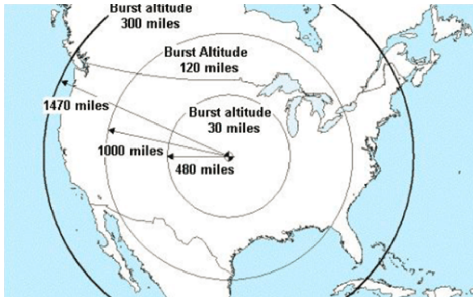
Figure 2-1 Burst Altitude and Impact Area
