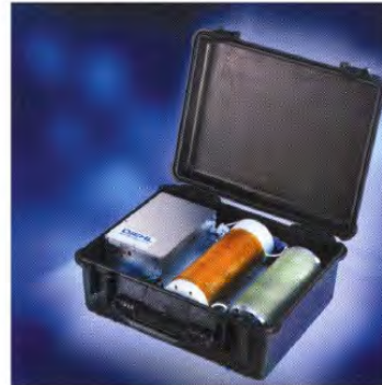
Figure 17. DIEHL Munitions damped sine IEMI generator
