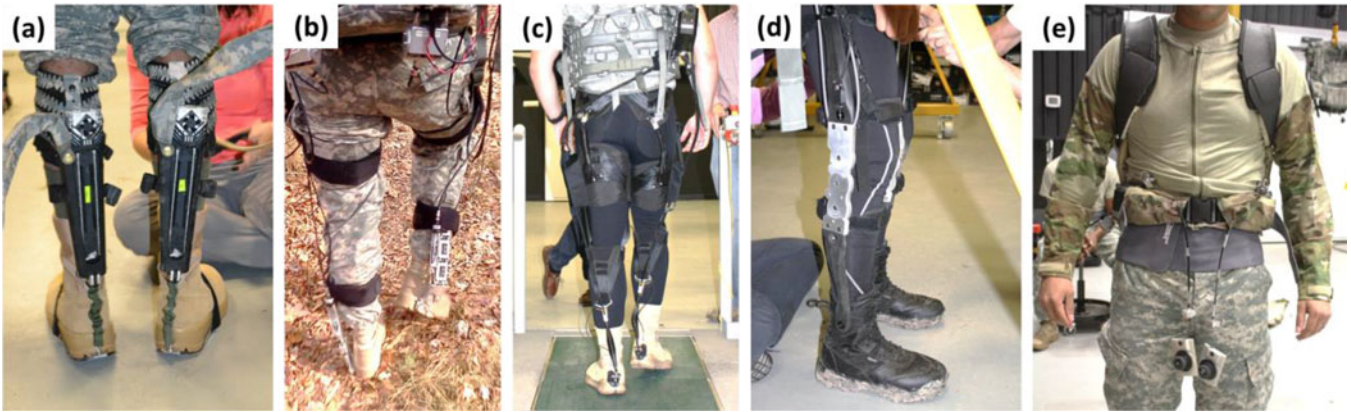
FIGURE 2 DARPA Warrior Web Task A Phase 2 prototypes: (a) Superflex exosuit by SRI, (b) Joint Torque Augmentation Robot (JTAR 2.0) by SpringActive, (c) Soft Exosuit by Wyss institute (Harvard University), (d) RheAct by Boston Dynamics/Eksobionics, and (e) UD WW system by University of Delaware.
