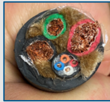
CCC cables contain three internal copper wire conduits and a smaller section of communication wires. CHAdeMO cables contain two internal copper wire conduits and three smaller sections of communications wires.
